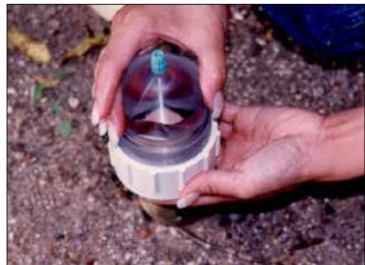
Photo 12 Tightening the Coupling
