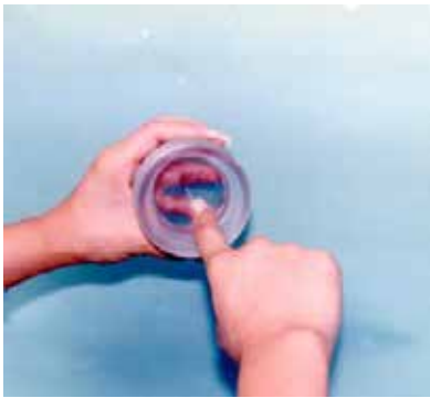
Photo 11 Greasing the Coupling
